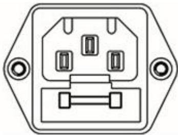
**Mains Fuse:** The mains fuse is located on the rear of the amplifier, just below the power cord socket (see picture on the left). The fuse rating is 1 x Littelfuse 213 Series 3.15A Slow Blow 5 x 20mm fuse for 100-125VAC and Littelfuse 213 Series 1.6A Slow Blow 5 x 20mm fuse for 200-250VAC. Always replace with the same type and value fuse! The fuse holder can be opened using a small slotted flat blade screwdriver.
