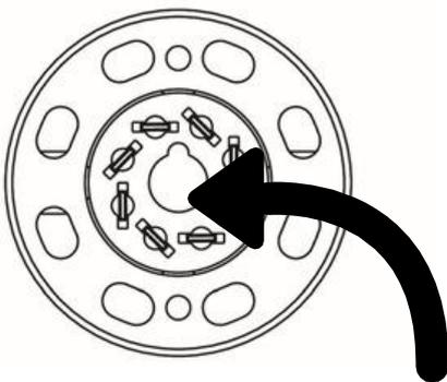
Some tubes and tube sockets have a "center key" which must line up! If you misalign them and use brute force, you will damage important and expensive parts of your amplifier!!
