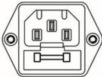
**Mains Fuse:** The mains fuse is located on the rear of the preamplifier, just below the power cord socket (see picture on the left). The fuse rating is 1 x Littelfuse 213 Series 1A Slow Blow 5 x 20mm fuse for 100-125VAC and Littelfuse 213 Series 0.5A Slow Blow 5 x 20mm fuse for 200-250VAC. Always replace with the same type and value fuse! The fuse holder can be opened using a small slotted flat blade screwdriver.
