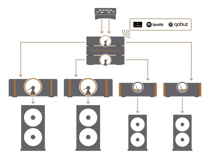
**To play the same source in Zone 1 and Zone 2 simultaneously:** Press the Zone 2 button and press the same input button that is active for Zone 1. The top chassis volume control functions as the Zone 1 volume control and the meter illumination remains green. The bottom chassis volume control now functions as the Zone 2 volume control and the meter is illuminated in a lighter green.
