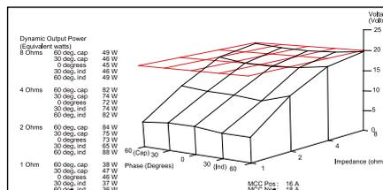
Despite its modest specs of 50 W, the Moonriver 404 is in fact over-spec'ed and doesn't reach the cube roof even at 8 Ω load. The result is still pretty good at 8 and 4 ohms, but after that the measurement drops off. Low but fairly symmetrical current on 16/18 amps.
